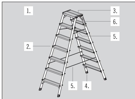
During the regular inspection of the ladder, inspection points 1-6 should be taken into account.
